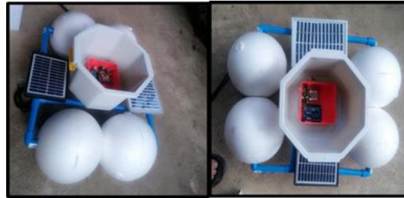
Figure 7. Smart WAMAS at first prototype coming from the sensors. This also has 3 sensor for pH, Turbidity and Temperature. It also has two solar panel that will be responsible for the power of the whole system and a motor cycle battery for energy storage.
